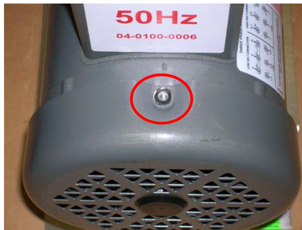
Figure 16 One of Three Screws on the Fan Shroud
