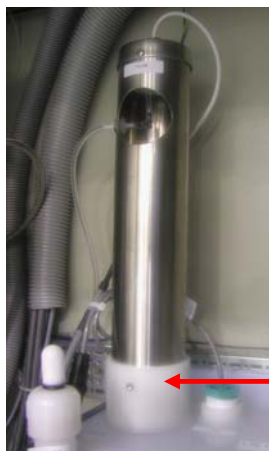
Figure 59 CG220 Oxygen Vent Tube
