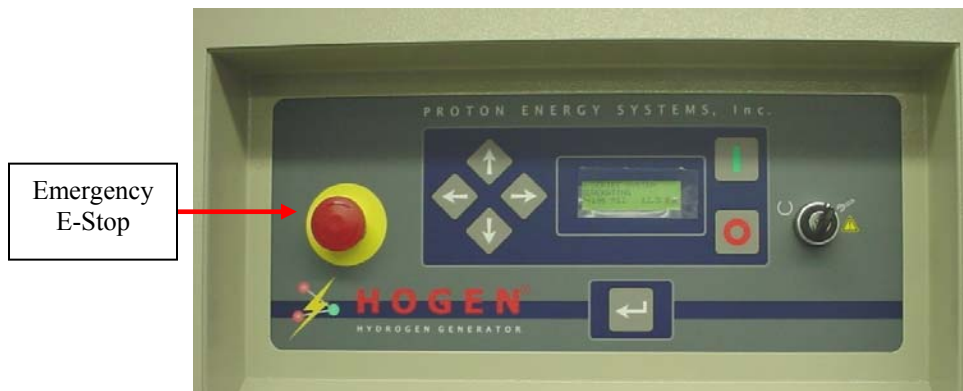
Figure 6 User Interface with Emergency E-Stop
