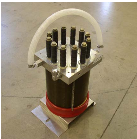
Figure 60 Hose Connected to the Inlet and Outlet of Cell Stack
