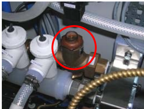
Figure 58 Temperature Control Valve Location
