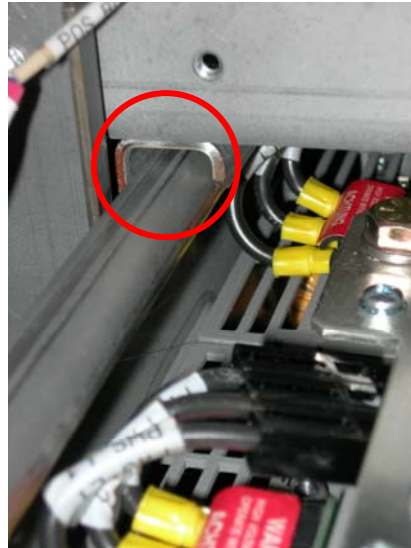
Figure 34 Support Rail Sliding into Power Supply Frame Track
