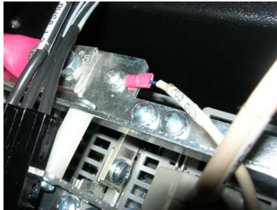
Figure 24 Removing Sense Lead Wires to the Bus Bars
