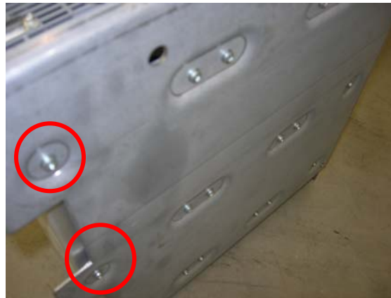
Figure 33 Location of Screws that Connect Power Supply to Support Plate
