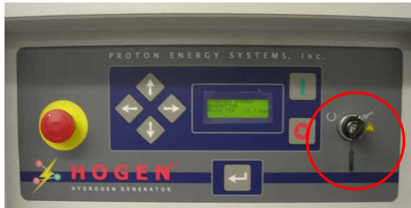
Figure 4 Key in Service Bypass Mode
