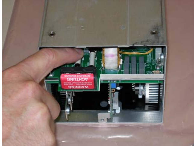
Figure 44 Snapping Fuses into Place
