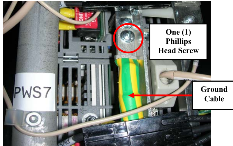
Figure 28 Ground Cable Location
