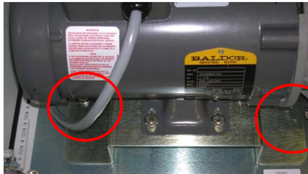
Figure 14 Two (2) Screws at Base of Pump Mounting Bracket
