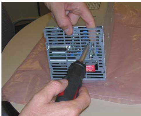
Figure 39 Removing the Screws from the Insulator
