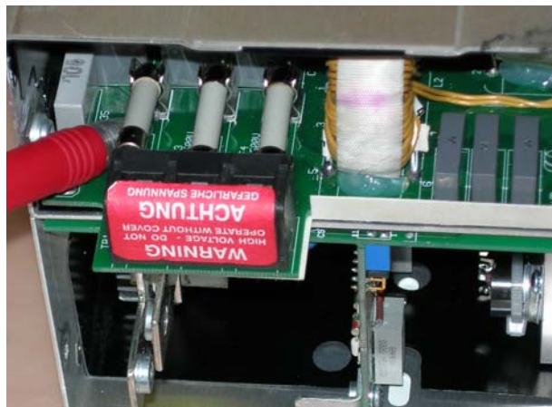
Figure 43 Removing the Fuses
